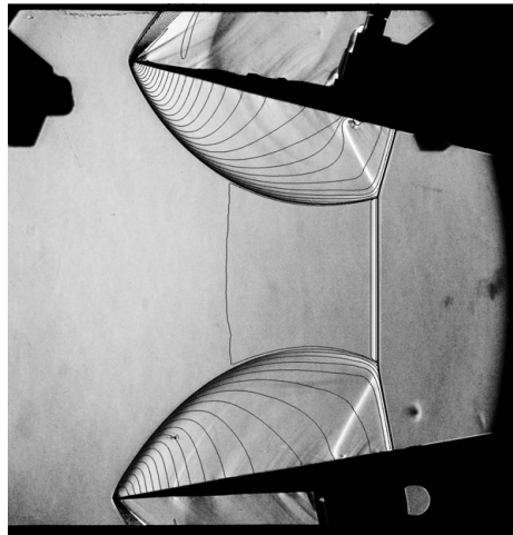
FIGURE 22. Comparison of schlieren and the simulation of shocks in \text{CO}_2 . The evidence of the relaxation zones is clear in both the schlieren and the pressure contours. Weak waves apparently originating on the wedge surfaces may be due to the roughness and limitations of the gaskets between the windows and the wedge.
